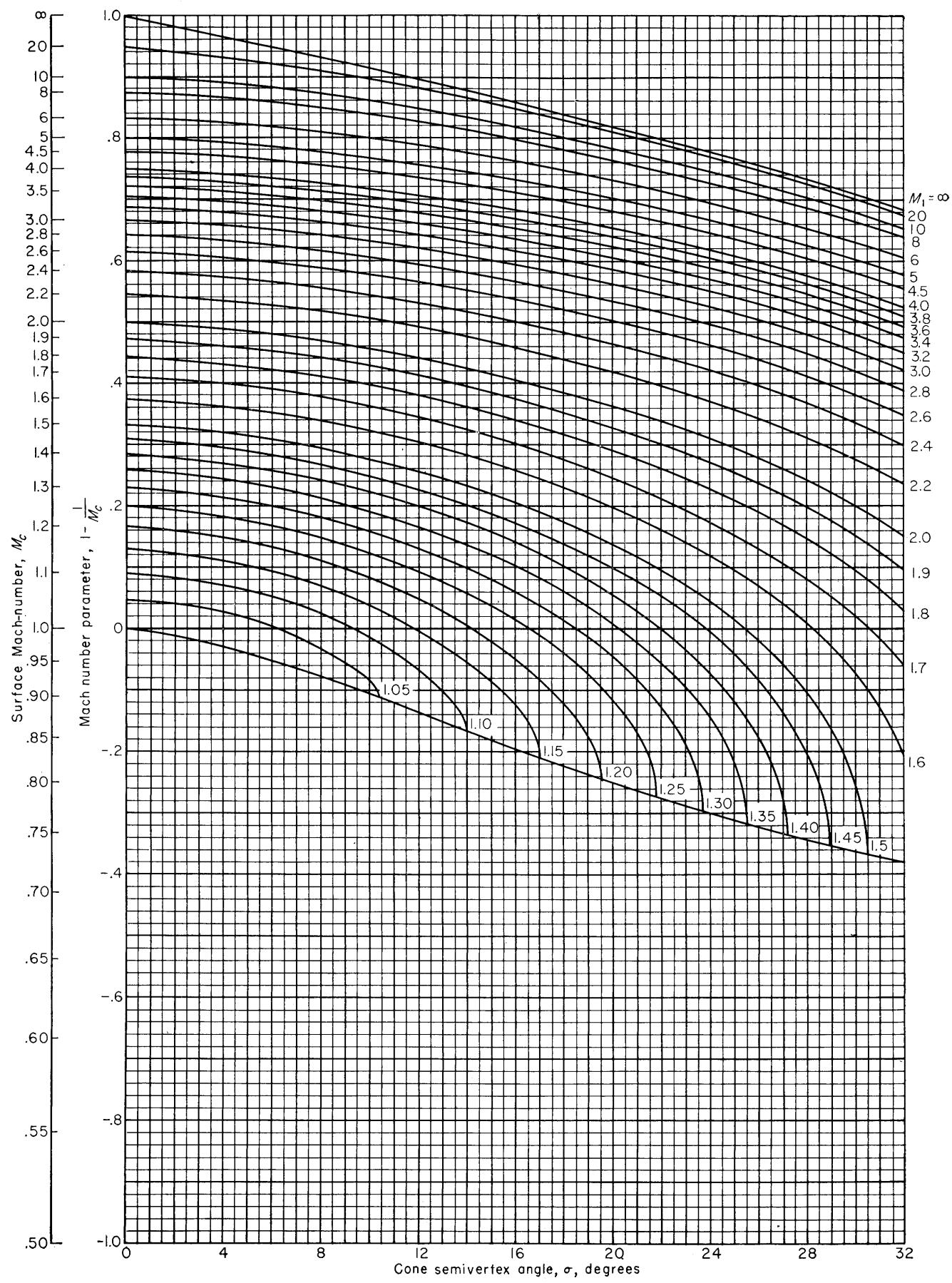
CHART 7.—Variation of Mach number at the surface of a cone with cone semivertex angle for various upstream Mach numbers. Perfect gas,
