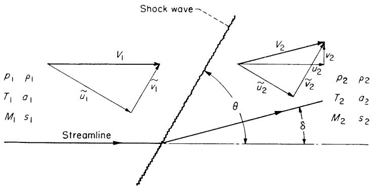
FIGURE 2.—Notation for oblique shock wave.
