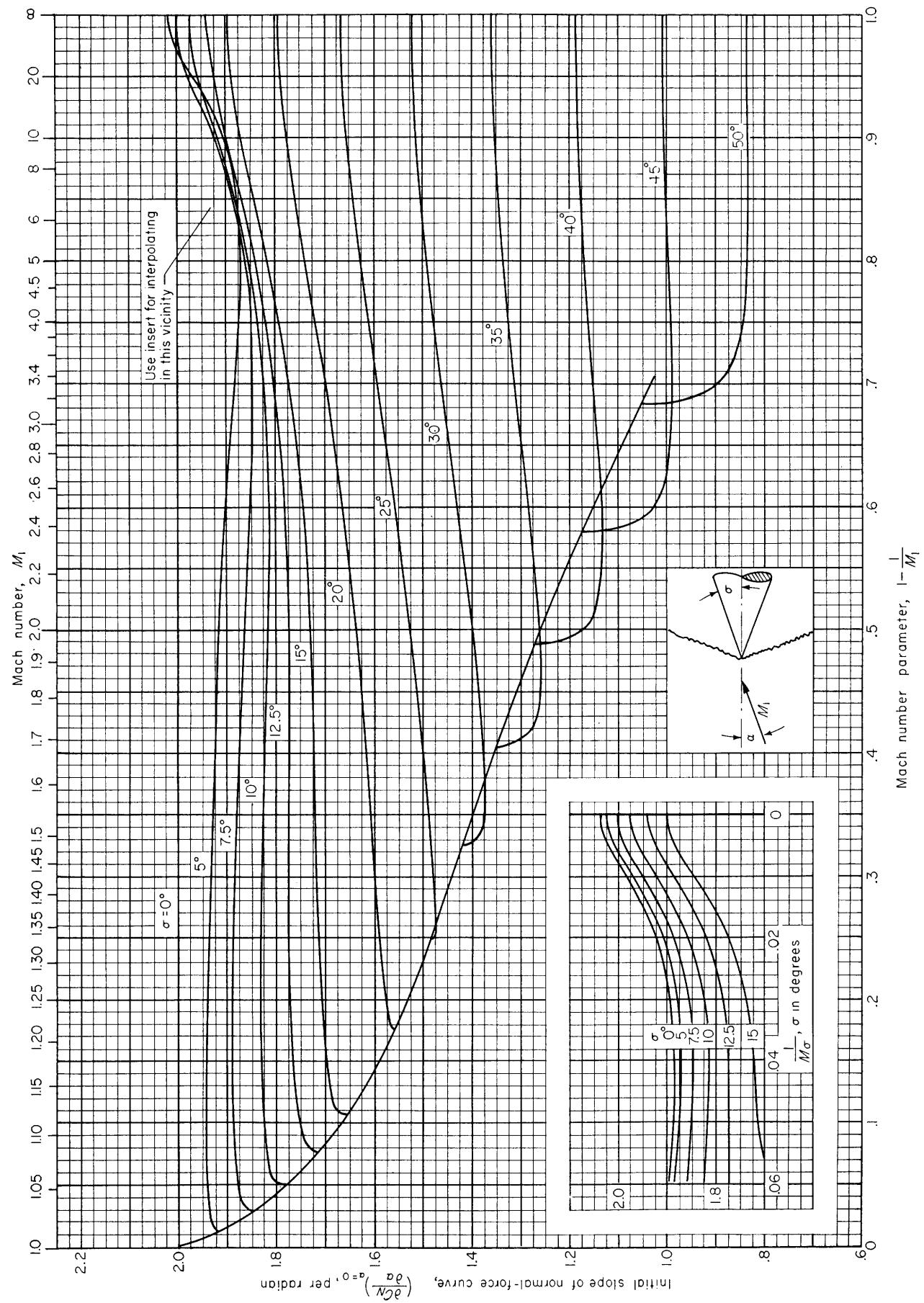
CHART 8.—Variation of the initial slope of the normal-force curve with upstream Mach number for various cone semivertex angles. Perfect gas,
