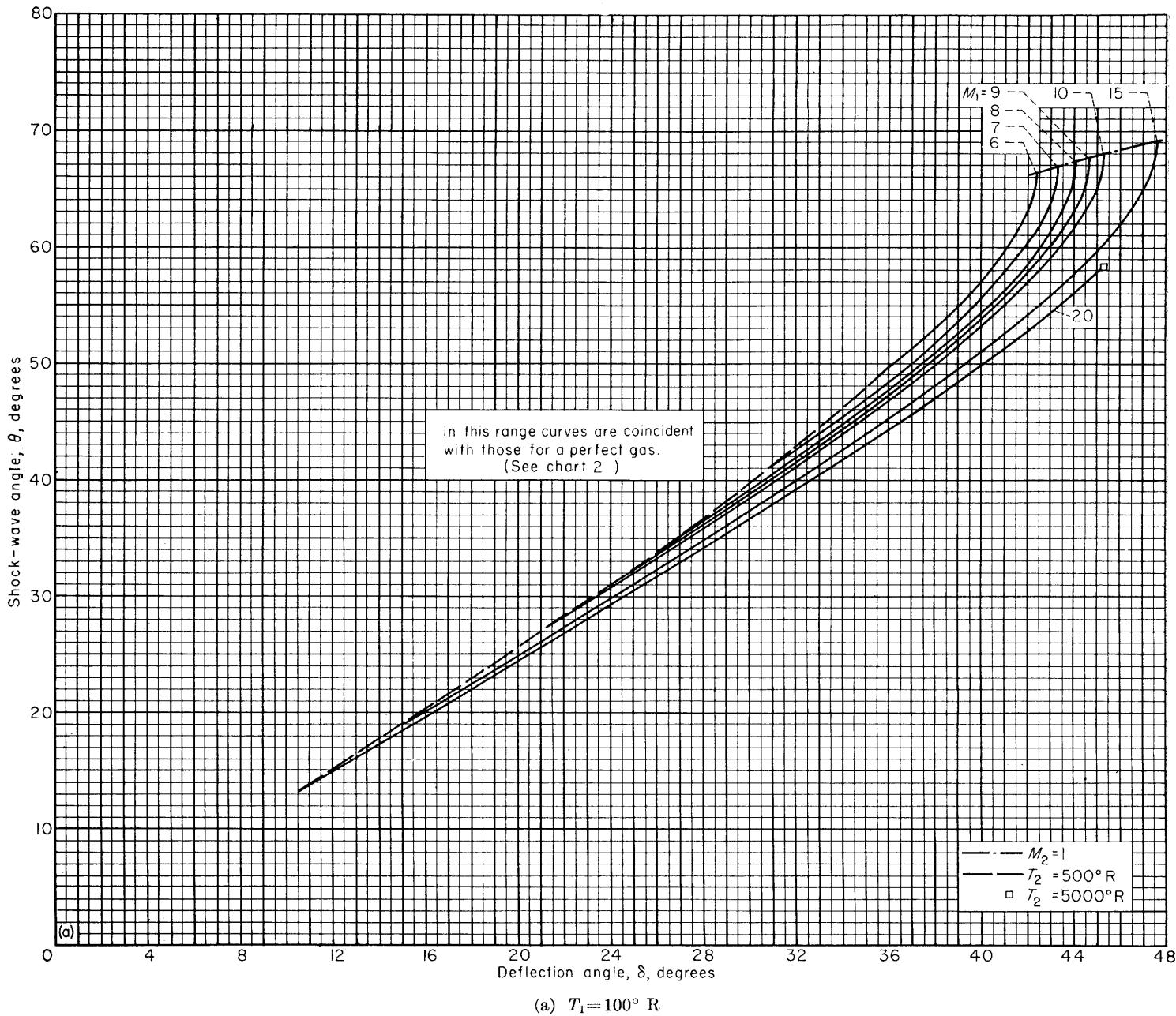
CHART 21.—Effect of calorific imperfections on the variation with flow-deflection angle of the shock-wave angle for a weak oblique shock wave.
