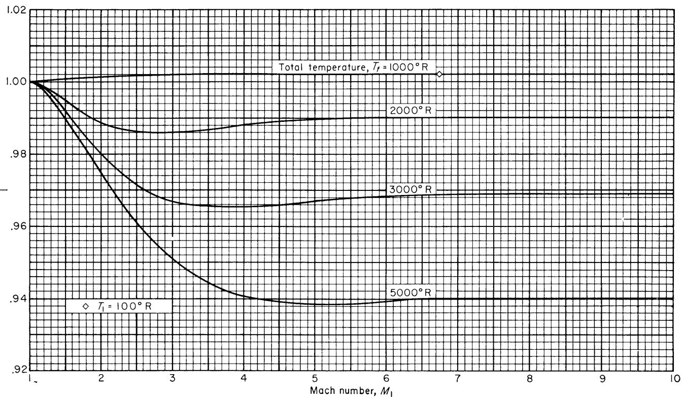
CHART 19.—Effect of caloric imperfections on the Mach number downstream of a normal shock wave.
