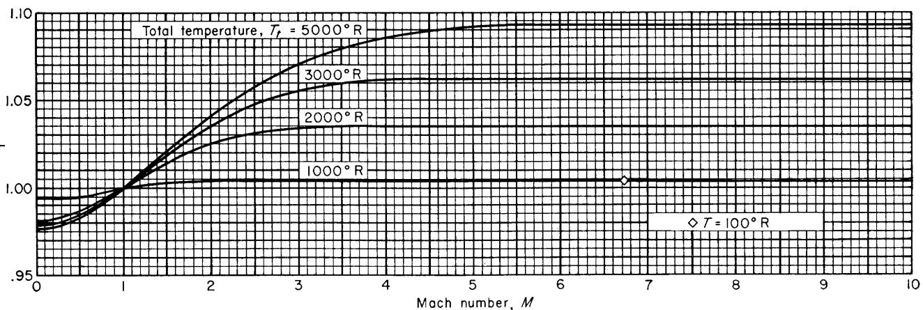
CHART 9.—Effect of caloric imperfections on the ratio of local speed to speed of sound at the point where  $M=1$ .
