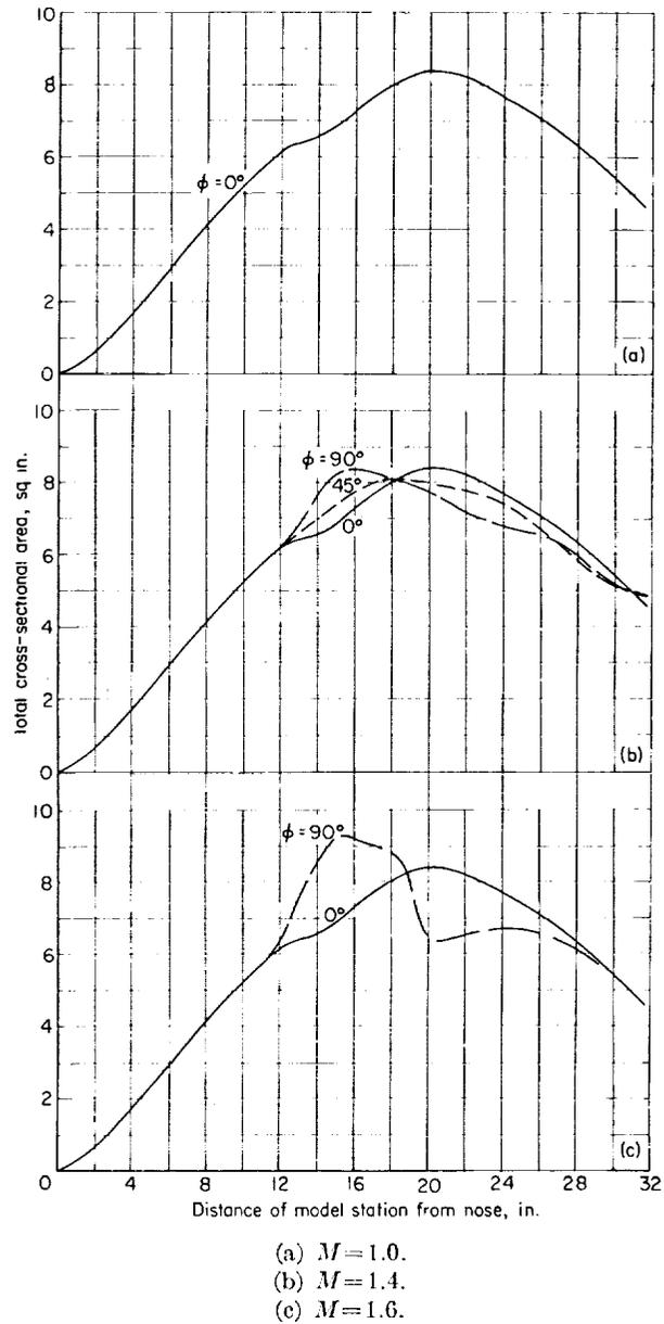
FIGURE 5.—Representative axial developments of cross-sectional area for the 60° swept wing in combination with the body indented for  $M=1.0$ , 1.4, and 1.6.
