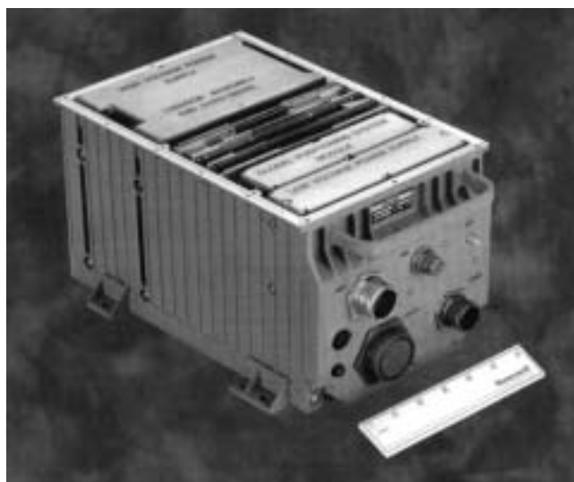
Wt = 22 lb Dimensions: 6 in. w × 8 in. × 12 in. lg (Honeywell)
